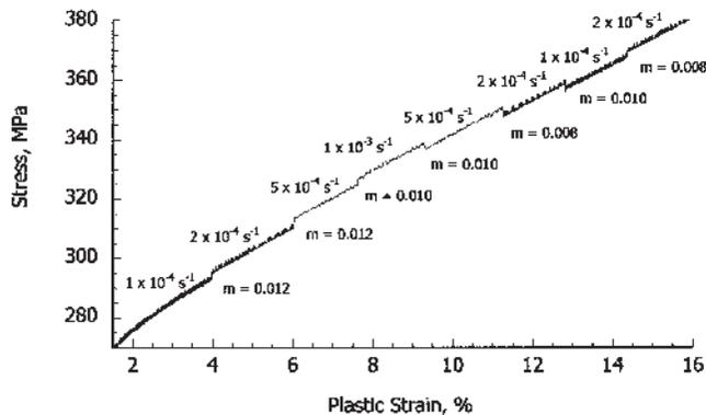
Fig. 5—Typical stress-strain trace (partial) illustrating the flow stress sensitivity on strain rate. As shown, a series of instantaneous strain-rate changes cause concomitant increases in flow stress. The resulting change in flow stress with a given change in strain rate is used to calculate the strain-rate-sensitivity,  $m$ .
