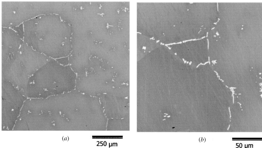
Fig. 1—(a) and (b) Microstructure of 52.5Ni-22.5Fe-25W, indicating that the composition slightly exceeds the solubility limit of tungsten in the 70Ni-30Fe base composition. Error bars represent  $\pm 1$  standard deviation.
