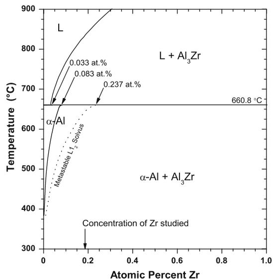
Fig. 7—Equilibrium Al-rich Al-Zr binary phase diagram (adapted from Murray<sup>[60]</sup>) with metastable  $\text{Al}_3\text{Zr}$  ( $\text{L}1_2$ ) solvus calculated by Liu *et al.*<sup>[61,62]</sup>
