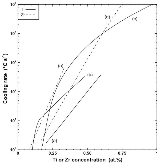
Fig. 8—Critical cooling rate for suppressing primary  $\text{Al}_3\text{Ti}$  (solid lines) or  $\text{Al}_3\text{Zr}$  (dashed lines) and achieving supersaturated  $\alpha\text{-Al}$  solid solution, as reported by (a) Ohashi and Ichikawa,<sup>[19]</sup> (b) Kerr *et al.*,<sup>[36]</sup> (c) Hori *et al.*,<sup>[75, 76]</sup> and (d) Hori *et al.*<sup>[24]</sup>
