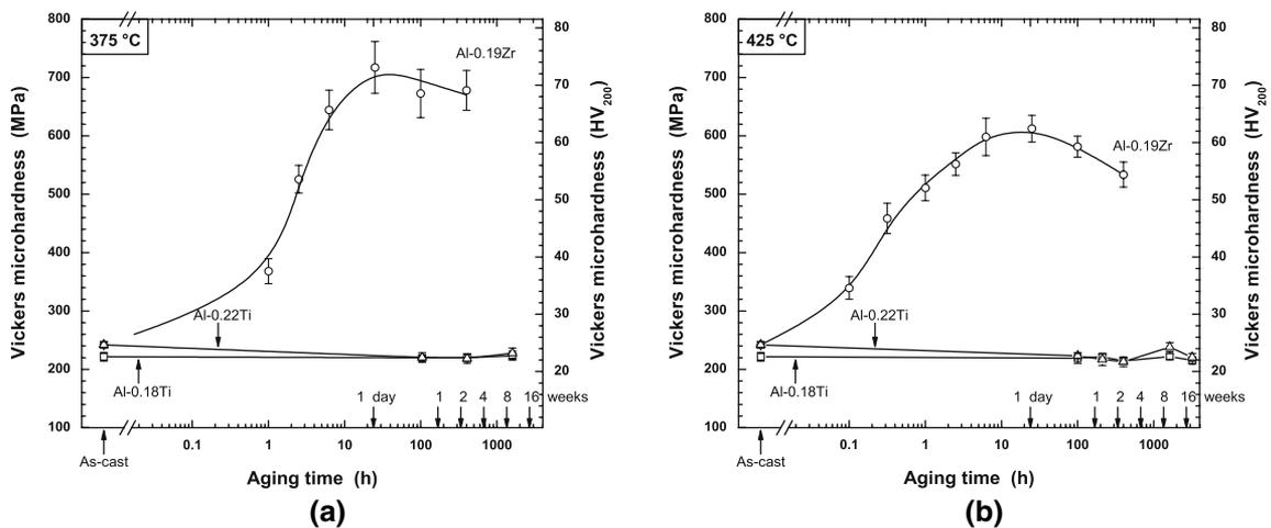
Fig. 3—Plot of Vickers microhardness vs aging time at (a) 375 °C and (b) 425 °C, for Al-0.18Ti, Al-0.22Ti, and Al-0.19Zr.
