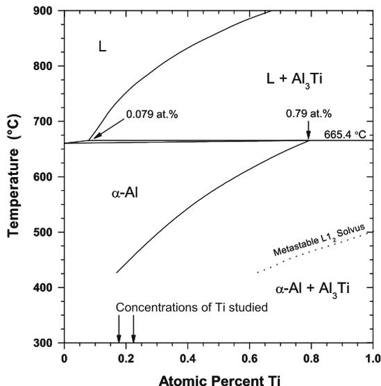
Fig. 6—Equilibrium Al-rich Al-Ti binary phase diagram (adapted from Murray<sup>[59]</sup>) with metastable  $\text{Al}_3\text{Ti}$  ( $\text{L}1_2$ ) solvus calculated by Liu *et al.*<sup>[61,62]</sup>
