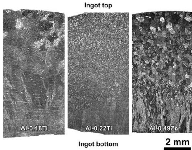
Fig. 1—Longitudinal cross sections of as-cast alloys Al-0.18Ti, Al-0.22Ti, and Al-0.19Zr, showing various degrees of grain refinement (etching with Poulton's reagent).
