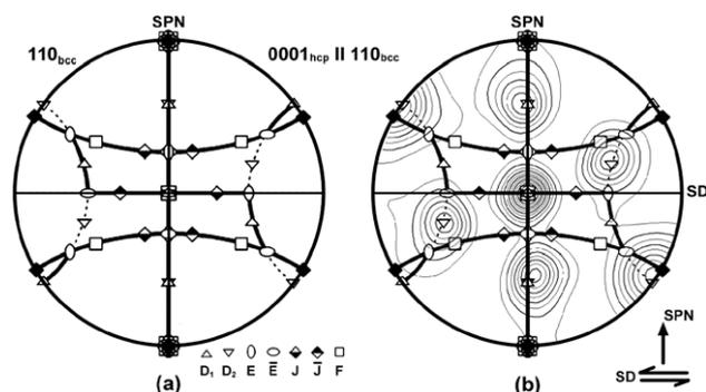
**Figure 3.** (a) Schematic  $\{110\}_{\text{bcc}}$  pole figure (in stereographic projection) showing the main texture component orientations and fibers associated with simple shear deformation of bcc metals (after Li et al. [28]). (b) Superposition of the  $\{110\}_{\text{bcc}}$  simple shear texture components on the  $\{0001\}_{\text{hcp}}$  pole figure of the deposited weld (rotated into the shear reference frame) from Figure 2(b).
