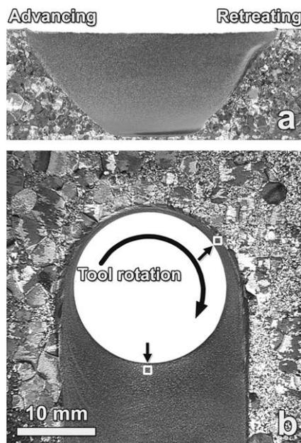
**Figure 1.** Transverse (a) and mid-thickness plan-view (b) cross-sections of the Ti-5111 friction stir weld. Approximate locations of the regions analyzed by EBSD are indicated by the arrowed regions in (b).
